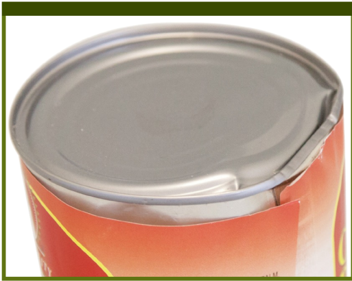
Severe dent in seam
